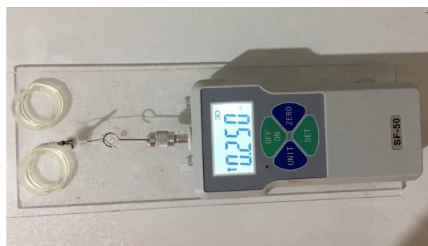
Figure 2. The force was measured using a digital force gauge.
