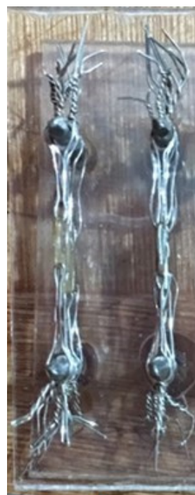
Figure 1. The two types of active tiebacks were stretched so that they exerted 250 g force initially at the 24 mm extension.
