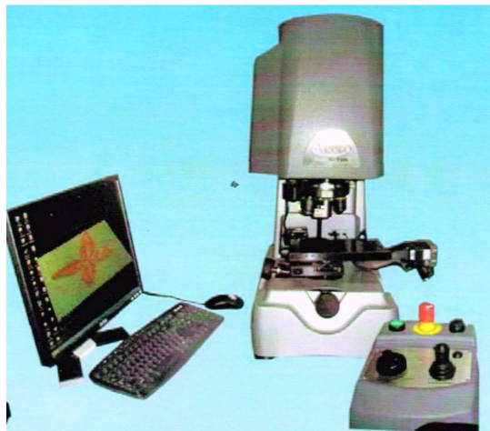
Fig. 1. 3D Profilometer used in the study for characterization of enamel surface changes
