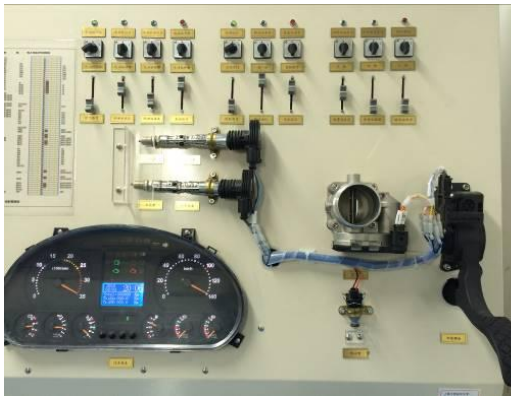
Fig. 13. Automatic test process of vehicle controller
