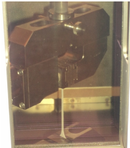
Fig. 8. Elongation of a specimen during testing at 140°C
