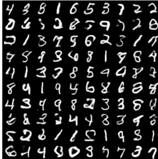
Figure 2. Images generated by sampling latent configurations with a quantum annealer that are subsequently transformed by a classical deconvolutional decoder. The classical networks and the quantum annealer weights have been trained end-to-end for 2000 epochs on the MNIST dataset using the quantum annealer as a sampler for estimating the gradients of the annealing parameters.
