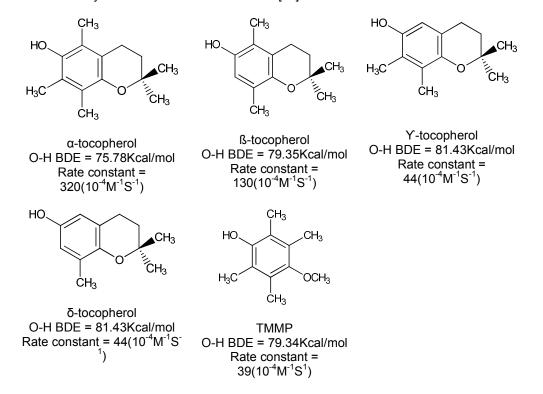
Fig. 4. Structures, O-H BDE and rate constants of tocopherols and TMMP [88]
