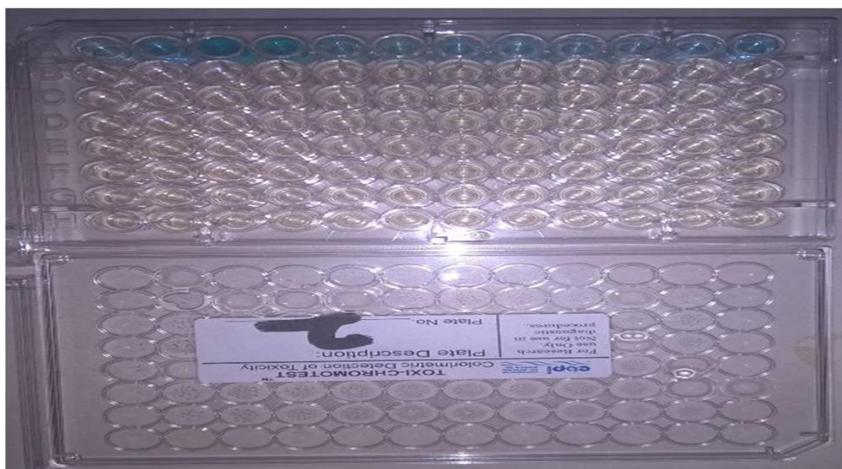
Plate 1. Microplate test result for Toxi - chromo testing of aromatic hydrocarbon compounds and marine water samples
