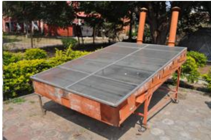
Fig. 1. Photographic view of NCSS dryer
