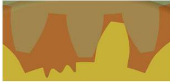
Fig. 5. Missing tooth profile
